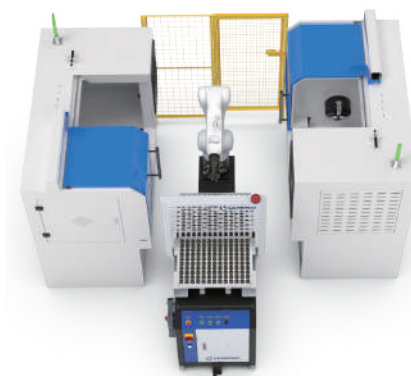
Double Production Rate 1 Robot - 2 Machine Setup
